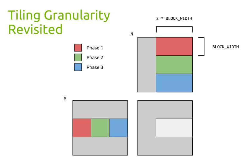
Tiles in Mare loaded redundantly by multiple blocks
