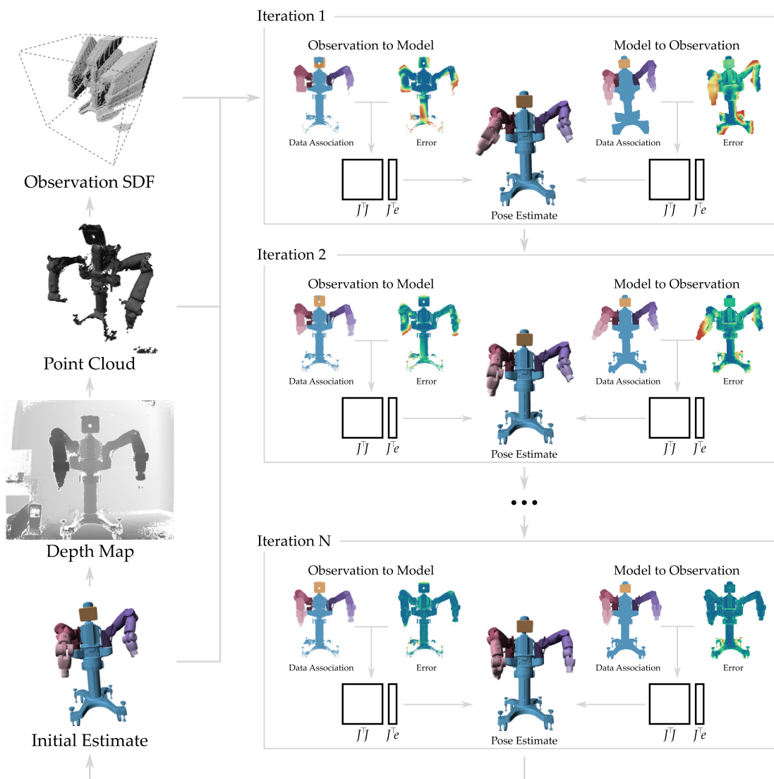
FIGURE 2.8: The flow of the DART tracking algorithm illustrated with a real instance of pose estimation for the Baxter robot. Starting with the initial estimate and depth map as input (lower left), we first compute the corresponding point cloud and observation SDF. We then iteratively refine the pose estimate, as shown on the right. The observation to model data association, the corresponding error, and the resulting normal equations can be computed in parallel with the model to observation data association, error, and normal equations. The normal equations are then combined to update the pose estimate. This process is repeated until convergence or until the next frame arrives. The final pose estimate along with its uncertainty is used as the initial pose estimate for the next frame, possibly after updating it through a dynamics model.
