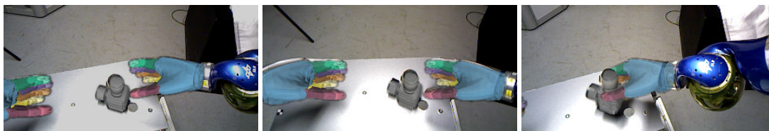
FIGURE 3.8: Tracking of the hands and object is maintained through changes in camera view. This allows the human operator to reposition the robot head (and thus the camera as well) for a more natural viewpoint on the manipulation.
