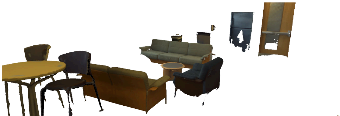
FIGURE 7.11: Objects detected by the object localization system described in section 7.3.2 in one of the held-out sequences. The video was recorded at night under artificial illumination, but the system localizes objects that were observed under many different lighting conditions.
